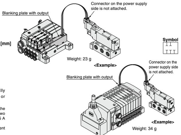
Blanking plate with a connector for individually outputting electricity to drive a single valve or equipment that are not on the manifold base.
