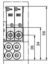
Mounted on the manifold block to make an independent exhaust port when the exhaust from one valve affects valves on other stations in the air circuit.
