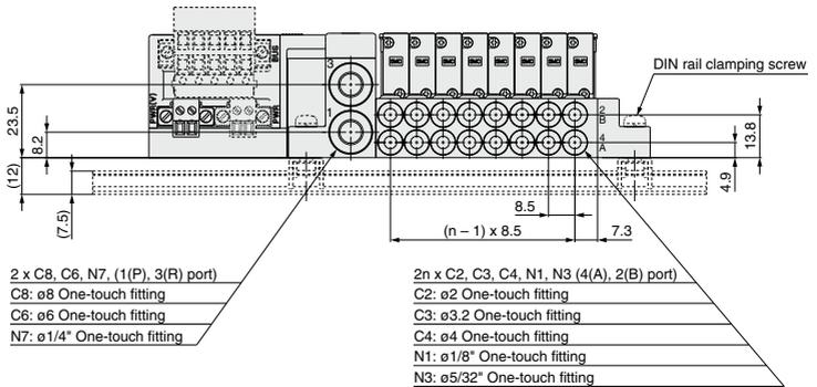
\*: Dotted line indicates DIN rail mounting bracket (-D).
