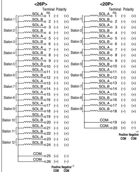
\*1: Mounting valve has no polarity. It can also be used as a negative common.
