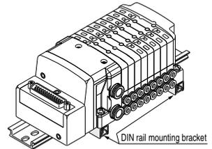
It is used for mounting a manifold on a DIN rail. The DIN rail mounted bracket is fixed to the manifold end plate. (The specification is the same as that for the option -D.) 1 set of DIN rail mounting bracket is included for 1 manifold (2 or 3 DIN rail mounting brackets (S, T kit)).
