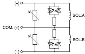
\*: Coil surge voltage generated when OFF is about -60 V. Please contact SMC separately for further suppression of the coil surge voltage.
