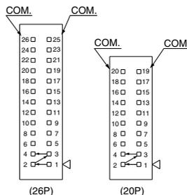
Mixed single and double wiring are available as an option. The maximum number of manifold stations is determined by the number of solenoids. Count one point for a single solenoid type and two points for a double solenoid type. The total number of solenoids (points) must not exceed 24 for 26P, 18 for 20P.
