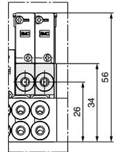
Mounted on the manifold block to make an independent supply port when each solenoid valve uses different operating pressure.
