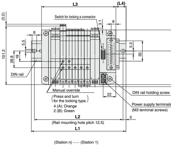
Applicable connector: {JIS-X-5101 } D-sub equivalent
