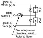
Note) Connect so that polarity is matched to the connector's (+), (-) and A, B and COM indicators. In case of voltage specifications other than 12 or 24 VDC, take care to avoid mistaking polarity, as there is no diode to prevent reverse current. In the event that lead wires are connected in advance, they will be as shown below.
