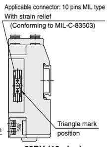
Note 1) Types 60PG and 60PH differ only in their connectors, and the L1 through L4 dimensions are the same as type 60P.
