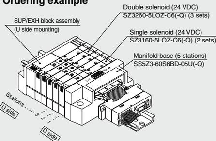
**SS5Z3-60S6BD-05U (-Q)**.....1 set (60S6B type 5-station manifold part no.)
