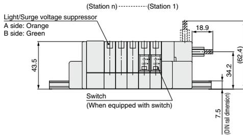
Internal Pilot Manifold L Dimension
