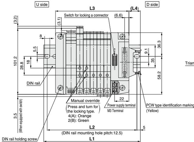
Applicable connector: 20 pin MIL type with strain relief (Conforming to MIL-C-83503)
