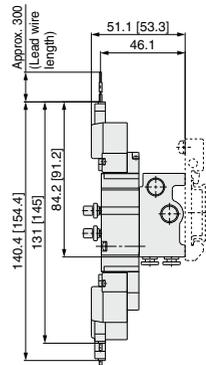
The dashed lines indicate the DIN rail mounting [-D].
