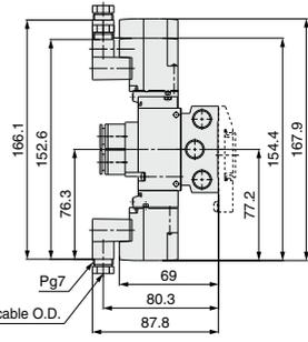
The dashed lines indicate the DIN rail mounting [-D].
