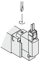
Push down completely on the manual override button with a small screwdriver. While down, turn clockwise 90° to lock it. Turn it counterclockwise to release it.
