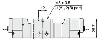
L-type plug connector (L): VQZ1  $\frac{3}{5}$  2  $\frac{0}{1}$  -□L□1-C3, C4, C6
