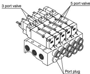
When port plug is used on 2 (B) port, indicate CM in manifold part no. and port size, and specify the port plug location by the manifold specification sheet.
