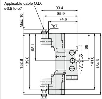
The dashed lines indicate the DIN rail mounting [-D]. Unless otherwise indicated, dimensions are the same as Grommet (G).
