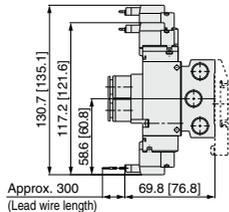
The dashed lines indicate the DIN rail mounting [-D].
