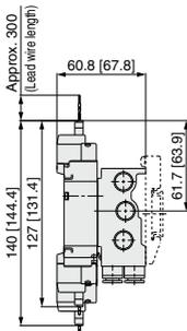
The dashed lines indicate the DIN rail mounting [-D]. Unless otherwise indicated, dimensions are the same as Grommet (G).
