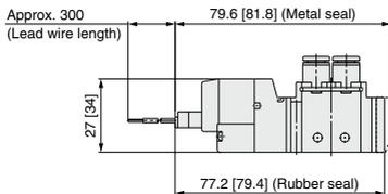
M-type plug connector (M): VQZ112<sup>0</sup> - □M□1-C3, C4, C6
