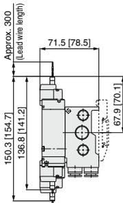
The dashed lines indicate the DIN rail mounting [-D].
