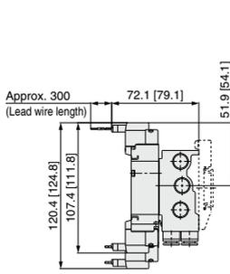
The dashed lines indicate the DIN rail mounting [-D]. Unless otherwise indicated, dimensions are the same as Grommet (G).
