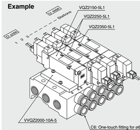
**VV5QZ25-05C6C** ... 1 set (C kit 5-station manifold base part no.)
