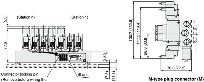
The dashed lines indicate the DIN rail mounting [-D].
