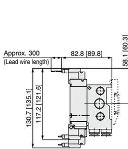
The dashed lines indicate the DIN rail mounting [-D].
