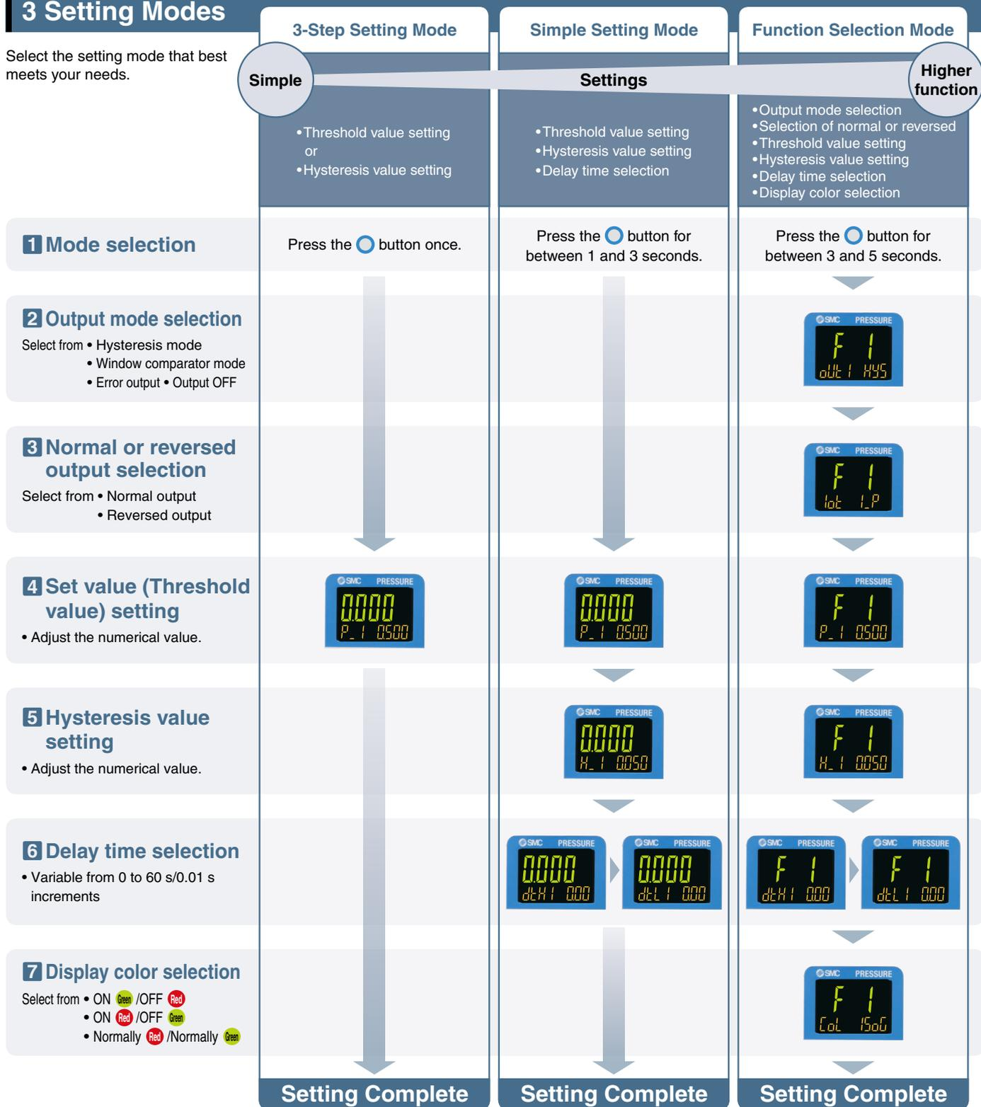
\* The chart above shows OUT1 operations. The Function Selection Mode for OUT2 is set using "F2." "2" will be displayed instead of "1" in the illustration above. (Example) P<sub>1</sub> → P<sub>2</sub>
