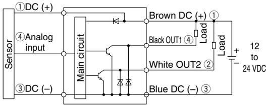
Setting of PNP open collector 2 outputs: Pressure sensor 3-wire type
