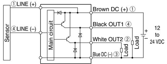
\* The output type can be changed in the function selection mode.
