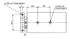
Note) 11-, 22-: Vacuum suction port Vacuum air from 2 ports on both sides. 10-/12-, 21-: Relief port Exhaust air from a port on one side. The port on the piston rod B side for 10-/12-, 21- is plugged since unlike the vacuum, it is not necessary to exhaust from 2 ports.
