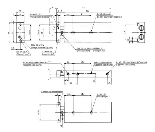
Note) 11-, 22-: Vacuum suction port Vacuum air from 2 ports on both sides. 10-/12-, 21-: Relief port Exhaust air from a port on one side. The port on the piston rod B side for 10-/12-, 21- is plugged since unlike the vacuum, it is not necessary to exhaust from 2 ports.
