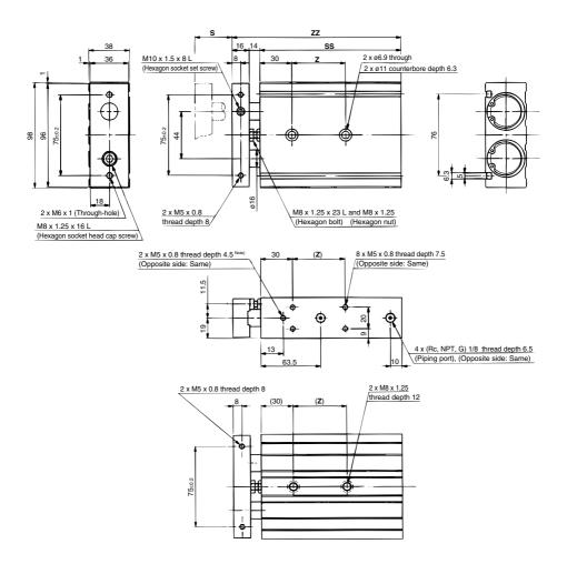
Note) 11-, 22-: Vacuum suction port Vacuum air from 2 ports on both sides. 10-/12-, 21-: Relief port Exhaust air from a port on one side. The port on the piston rod B side for 10-/12-, 21- is plugged since unlike the vacuum, it is not necessary to exhaust from 2 ports.
