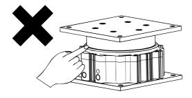
4. Do not bring objects that are sensitive to magnetism near the cylinder.
