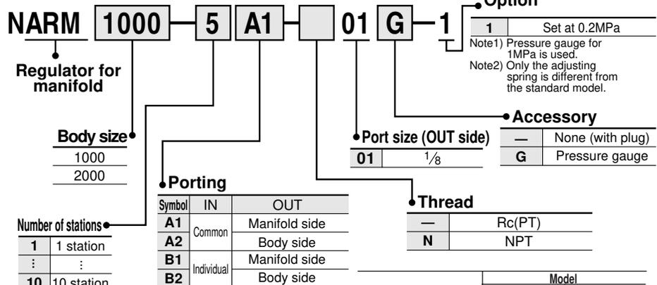
Note1) In case of A1 and B1, a pressure gauge or a plug is mounted at the body side, while in case of A2 and B2, at the manifold side.
