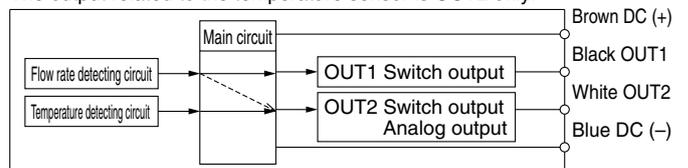
The OUT2 can be selected from either the output for temperature or flow rate by button operation.
