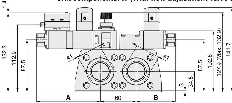
Supply unit Unit components: S (With flow adjustment valve)
