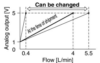
For 4 L/min type (Integrated display)
