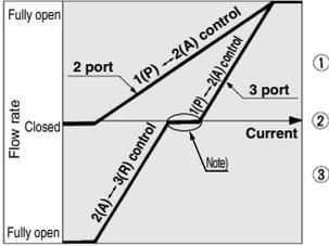
Note) The areas between port 1 (P) and 2 (A) and between port 2 (A) and 3 (R) will not equal the effective area of 0 mm<sup>2</sup> (valve closed) at the same time. (Refer to the flow characteristics.)
