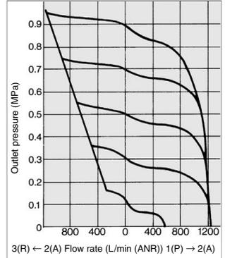
**Pressure Characteristics** JIS B 8372 (In accordance with air regulator)
