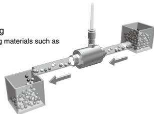
\* SMC does not guarantee the entire system. Please think the system shown above as an example. A workpiece that is harder than the body material (aluminum alloy) may damage to the inside of the body, causing the performance to lower. The compatibility should be judged by the customer before adopting the product.
