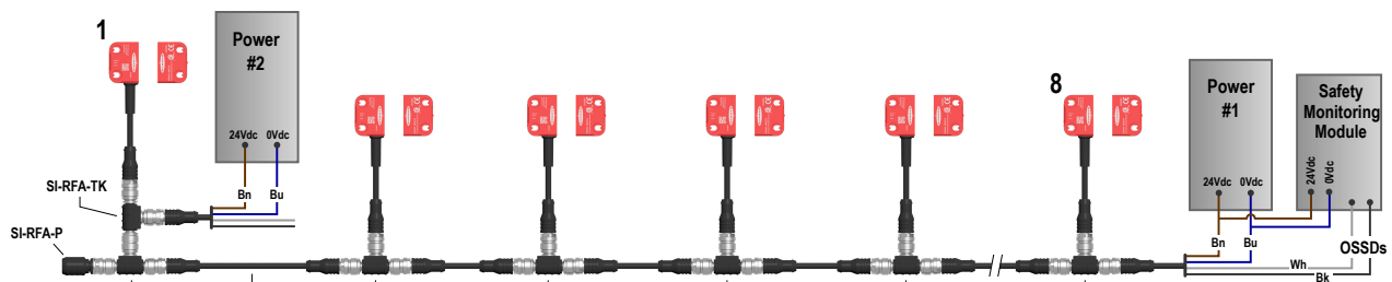
Figure 8. Option 1: Use a SI-RFA-TK Reset Connector in series with ISD Device. If available, set the power supplies for parallel output.
