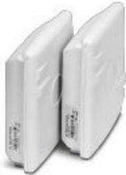
Pre-configured point-to-point Ethernet bridge kit for USA and Canada with internal antennas for pole mounting (outer dimensions 0.25 in. to 2 in.). IP67, wireless Ethernet communication up to 300 Mbps, frequency: 2.4 GHz, 10/100/1000 Mbps RJ45, passive PoE powered.
