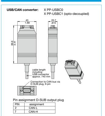
This is a metric design and millimeter dimensions take precedence. Applicable for nominal dimensions without direct tolerance indication: DIN ISO 286 ± IT 13.
