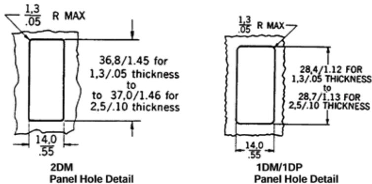
This Honeywell datasheet supports the following MICRO SWITCH™ DM & DP Series Basic Switch Listings
