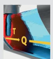
**Temperature measurement** The calorimetric principle allows the permanent measurement of the media temperature in addition to the flow. The user thus receives valuable additional information. A separate device is no longer required to measure the temperature.
