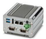
IP30-rated fanless industrial box PC (BPC) with energy-efficient Intel® Celeron® N3350 processor with 32 GB eMMC mass storage, 128 GB M.2 SSD, 2x COM ports, Windows 10 Enterprise 2019 LTSC operating system, and a Trusted Platform Module (TPM)
