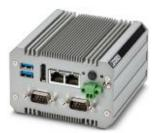
IP30-rated fanless industrial box PC (BPC) with energy-efficient Intel® Celeron® N3350 processor with 32 GB eMMC mass storage, 64 GB M.2 SSD, 2x COM ports, Windows 10 Enterprise 2019 LTSC operating system, and a Trusted Platform Module (TPM)
