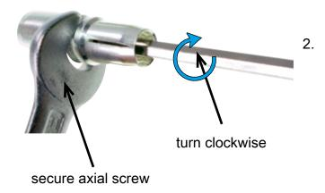
Please insert suitable torque key (SW 4) into the contact from mating side and turn the axial screw clockwise. For that purpose secure the axial screw with a spanner (SW 11).
