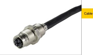
Identification Part number Drawing Dimensions in mm har-speed M12 PFT with cable with 0.3 m cable "Cat. 7<sub>A</sub> (2 x AWG 27/7) PIMF". 21 33 080 0850 003 Other lengths on request with 0.3 m cable "HA-VIS EtherRail Cat. 7 4 x (2 x AWG 24/7)". 21 33 070 0853 003 Other lengths on request
