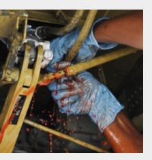
It's not a matter of *if* but *when* hydraulic systems will leak or break. Clean-up is messy and time-consuming. When hydraulics fail, the production parts/product may need to be scrapped out and production stopped while repairs and cleanup are undertaken.
