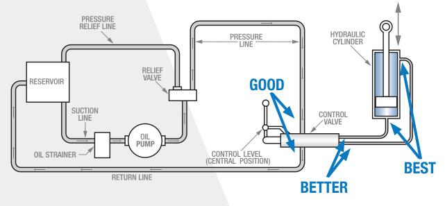
The next best and most practical way is to measure hydraulic pressures in the cylinder while the process is in operation.
