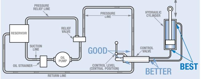
This diagram shows the preferred locations to measure pressure to accurately determine the actual force required in an existing application
