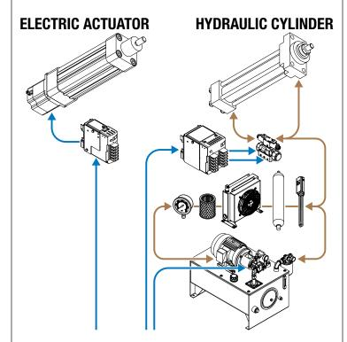
Hydraulic cylinders and required components are more complex than electric actuators
