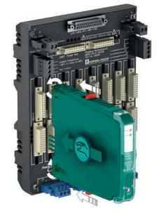
Installation of power and diagnostic modules works without tools Figure 13
