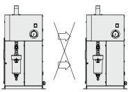
Confirm that the exhaust air does not flow into the neighboring equipment.
