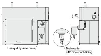
\* The heavy-duty auto drain and piping materials (nipple, elbow) are shipped together with the main body of the air dryer. Customers are required to mount the parts to the air dryer.
