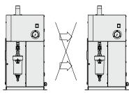
Confirm that the exhaust air does not flow into the neighboring equipment.
