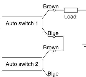
When two auto switches are connected in series, a load may malfunction because the load voltage will decline when in the ON state. The indicator lights will light up when both of the auto switches are in the ON state. Auto switches with a load voltage less than 20 V cannot be used.
