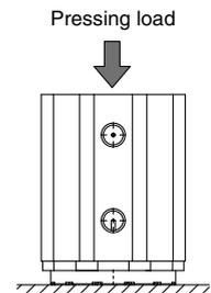
5. Do not apply impact load to the center of the magnetic attraction surface.
