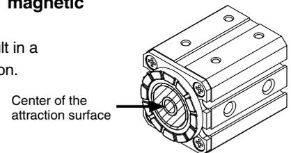
6. The head cap is magnetized during the release of workpiece. Iron particles may be attracted.
