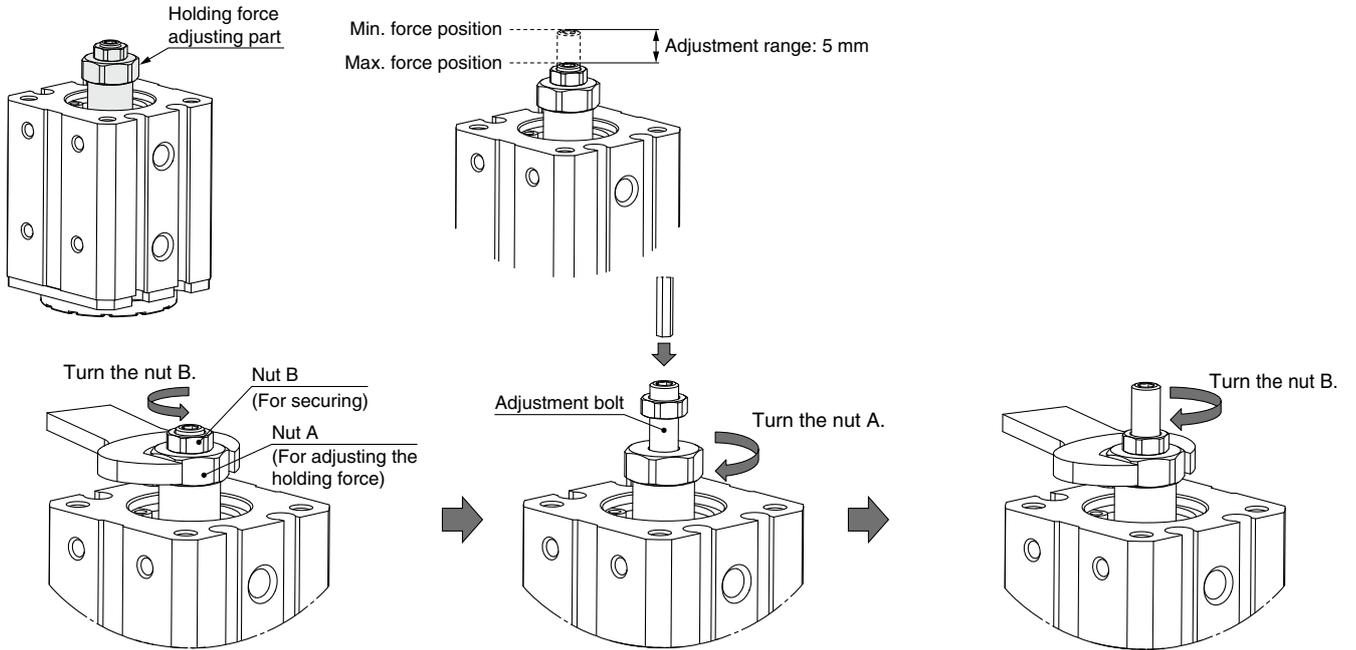
1. Turn the nut B to loosen while holding the nut A. (Nuts are tightened to a specified torque around the maximum holding force position (zero adjustment).)
