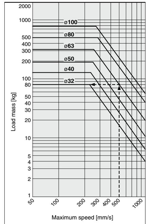
Example) Load limit at rod end when the air cylinder ø63 is actuated at 500 mm/s.
