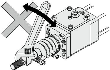
4. Do not disassemble the trunnion type cylinder because the mounting precision is required.
