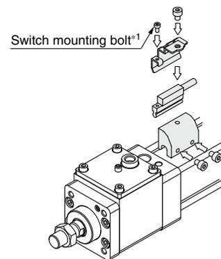
\*1 The switch mounting bolt is supplied with the switch.
