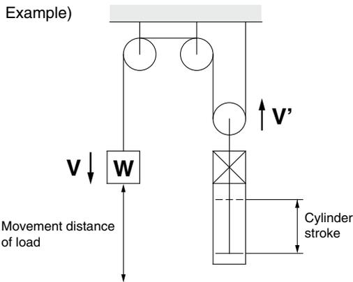
3. The following selection example and procedures are based on use at the intermediate stop (including emergency stops during operation). However, when the cylinder is in a locked state, kinetic energy does not act upon it. Under these conditions, use the load mass at the maximum speed ( $V$ ) of 100 mm/s shown in graphs [5] to [7] on page 6 depending on the operating pressure and select models.
