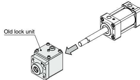
4) Insert a new lock unit into the cylinder. The lock unit for maintenance is supplied with lock released state at the shipment from the factory.
