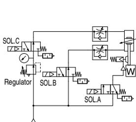
[Load in the direction of rod retraction]
