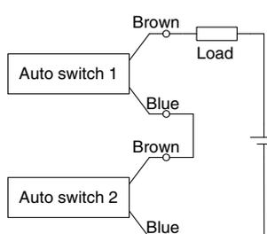
When two auto switches are connected in series, a load may malfunction because the load voltage will decline when in the ON state. The indicator lights will light up when both of the auto switches are in the ON state. Auto switches with a load voltage less than 20 V cannot be used.
