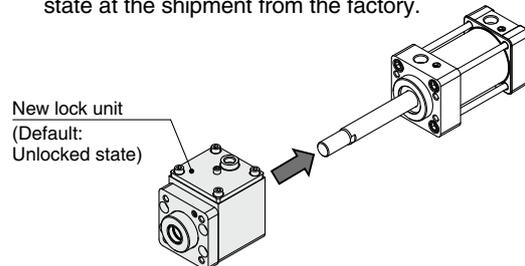
5) Insert the lock unit holding bolt and tighten it temporarily. Check that the piston rod operates smoothly by hand while maintaining the lock released state.
