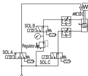
\* The symbol for the cylinder with lock in the pneumatic circuit uses SMC original symbol.
