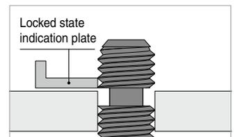
\* If the bolt is not sufficiently turned counterclockwise, the groove position will not be aligned and the locked state indication plate cannot be inserted.
