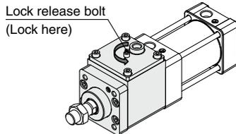
Check that the cylinder is locked and confirm that the lock is released when air pressure of 0.3 MPa or more is applied to the unlock port on the lock unit. In addition to this, the piston rod should operate smoothly with the minimum operating pressure. Check that there is no air leakage from the lock release bolt.
