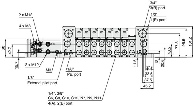
Note) The dimensions of the bottom ported type are common to all S kits.
