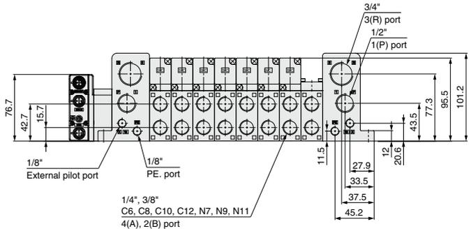
Note) The dimensions of the bottom ported type are common to all S kits.
