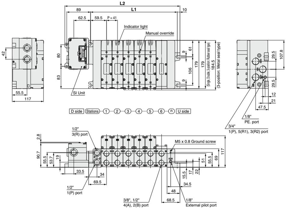
Note) The dimensions of the bottom ported type are common to all S kits.
