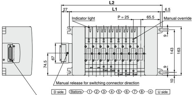
Applicable connector: D-sub connector (25P)
