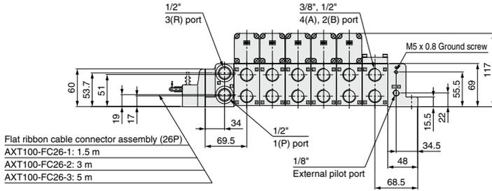
Flat ribbon cable connector assembly (26P)
