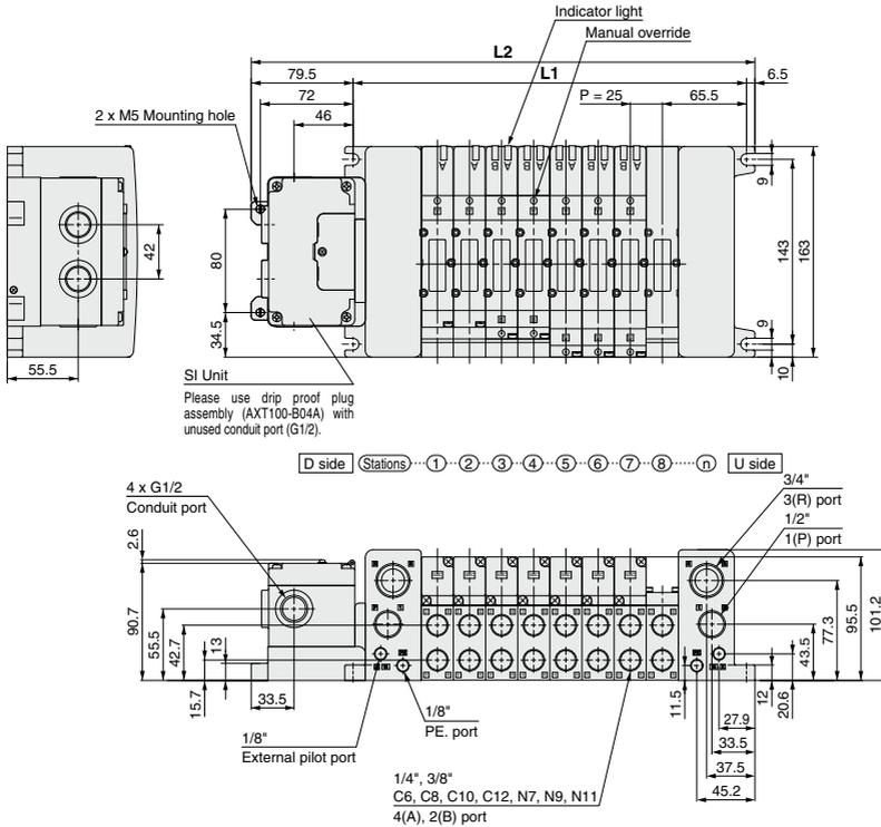
Note) The dimensions of the bottom ported type are common to all S kits.
