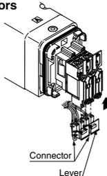
Note) Do not pull on the lead wires with excessive force. This can cause faulty and/or broken contacts.
