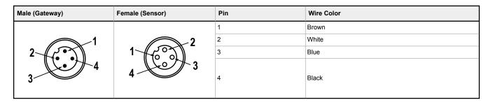
**Important:** If using a cable to connect the converter to an analog sensor, use of a shielded M12 cable is recommended, with the shield tied to pin 3.
