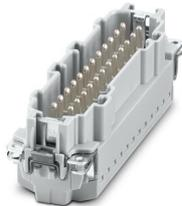
Contact insert, number of positions: 24+2 PE, size: B24, number of connections per position: 1, Pin, Push-in connection, 500 V, 16 A, 0.14 mm<sup>2</sup> ... 2.5 mm<sup>2</sup>, application: Power, tool-free Click-in mounting
