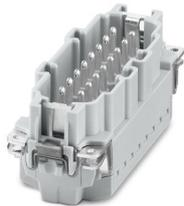
Contact insert, number of positions: 16+2 PE, size: B16, number of connections per position: 1, Pin, Push-in connection, 500 V, 16 A, 0.14 mm<sup>2</sup> ... 2.5 mm<sup>2</sup>, application: Power, tool-free Click-in mounting
