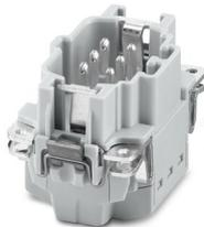
Contact insert, number of positions: 6+2 PE, size: B6, number of connections per position: 1, Pin, Push-in connection, 500 V, 16 A, 0.14 mm<sup>2</sup> ... 2.5 mm<sup>2</sup>, application: Power, tool-free Click-in mounting
