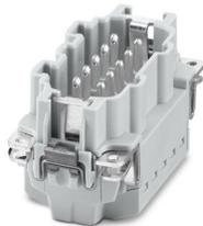
Contact insert, number of positions: 10+2 PE, size: B10, number of connections per position: 1, Pin, Push-in connection, 500 V, 16 A, 0.14 mm<sup>2</sup> ... 2.5 mm<sup>2</sup>, application: Power, tool-free Click-in mounting
