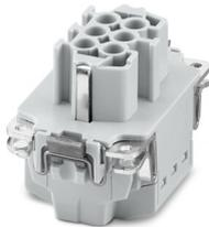
Contact insert, number of positions: 6+2 PE, size: B6, number of connections per position: 1, Socket, Push-in connection, 500 V, 16 A, 0.14 mm<sup>2</sup> ... 2.5 mm<sup>2</sup>, application: Power, tool-free Click-in mounting
