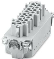
Contact insert, number of positions: 16+2 PE, size: B16, number of connections per position: 1, Socket, Push-in connection, 500 V, 16 A, 0.14 mm<sup>2</sup> ... 2.5 mm<sup>2</sup>, application: Power, tool-free Click-in mounting
