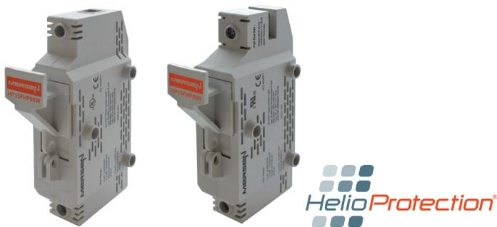
Mersen's 1500VDC HelioProtection fuse holders for 20x65mm PV fuses introduce the next level of safety for higher amperage utility-scale photovoltaic applications. The HP15FHP80 fuse holders are finger safe (IP20 ingress protection rated) and feature a rotating fuse carrier like the Mersen UltraSafe® fuse holders.
