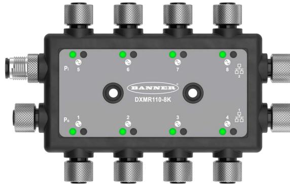
The DXMR110-8K contains eight IO-link ports, allowing for concurrent communication to up to eight IO-Link devices. Data is collected into the internal logic controller to facilitate edge processing, protocol conversion to Industrial Ethernet, Modbus/TCP, and PROFINET, and pushing information to web servers. In addition to IO-Link devices, the IO-Link master can be used to transmit up to 16 discrete signals using pin 2 or pin 4 of the IO-link master ports.
