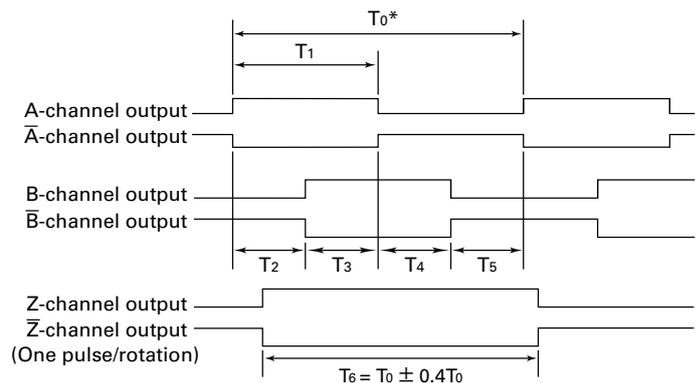
\* $T_0$  is the average time for one encoder rotation when the encoder is rotated at a constant speed.
