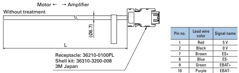
Compatible motors: R2CA2830KV, R2CA3255KB for EtherCAT and built-in positioning type servo amplifiers
