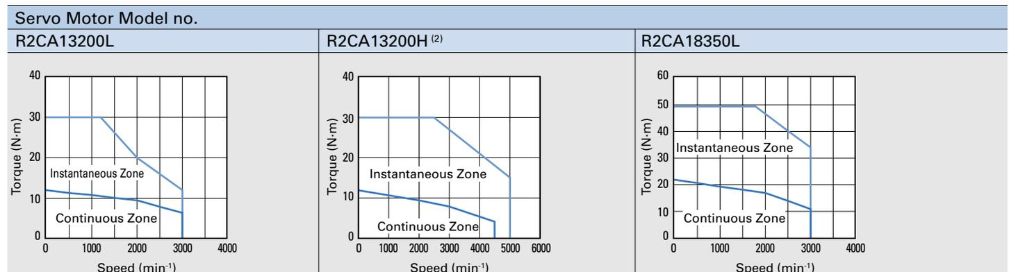
(2) Operate a motor so that the average speed does not exceed its maximum speed in the continuous zone.
