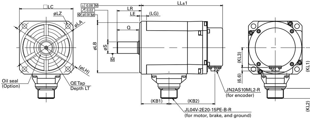
This dimensional drawing is for a servo motor equipped with a battery-less absolute encoder and a brake.
