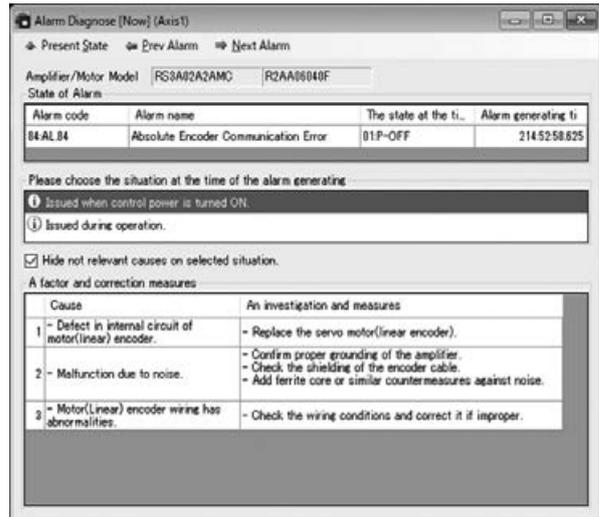
Causes and corrective actions can be checked based on alarm status.
