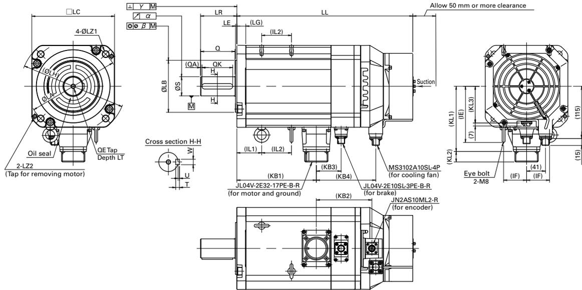
This dimensional drawing is for a servo motor equipped with a battery-less absolute encoder and a brake.
