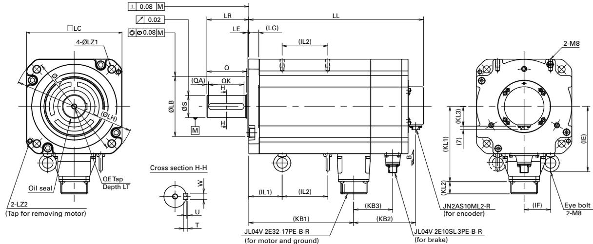
This dimensional drawing is for a servo motor equipped with a battery-less absolute encoder and a brake.
