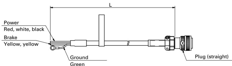
Connect power line to the servo amplifier's connector CNB.
