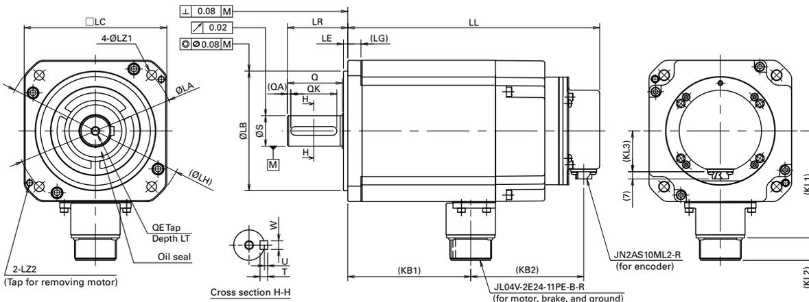
This dimensional drawing is for a servo motor equipped with a battery-less absolute encoder and a brake.
