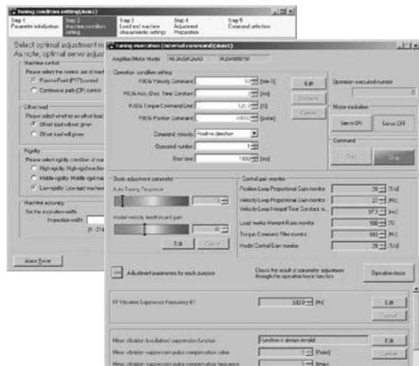
By setting the mechanical conditions, servo tuning can be easily made with the optimal tuning mode.
