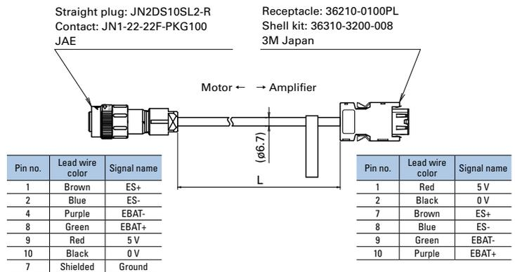
Compatible motors: Other than R2CA2830KV, R2CA3255KB, for EtherCAT and built-in positioning type servo amplifiers
