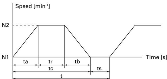
$N_1$ : Servo motor rotational speed before acceleration [ $\text{min}^{-1}$ ]
