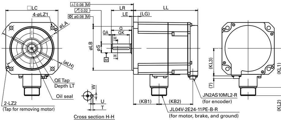
This dimensional drawing is for a servo motor equipped with a battery-less absolute encoder and a brake.
