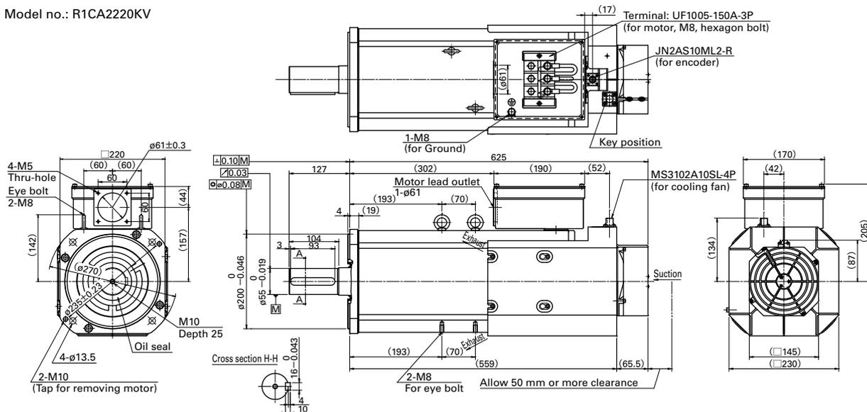
This dimensional drawing is for a servo motor equipped with a battery-less absolute encoder and no brake.
