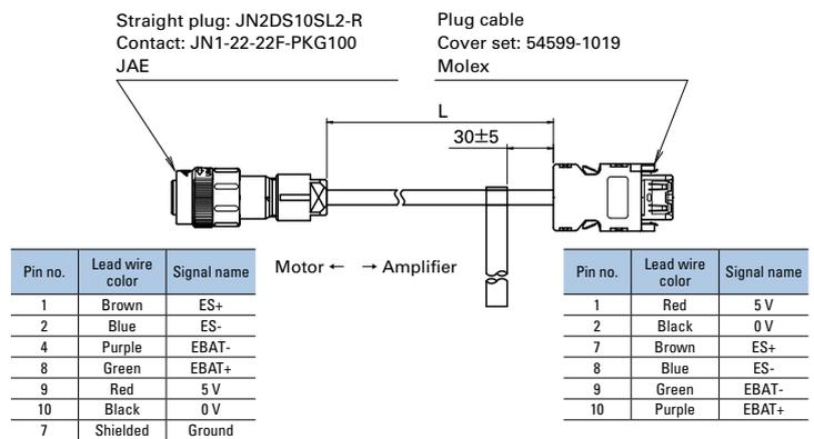
Compatible motors: R2CA2830KV, R2CA3255KB for analog/pulse type servo amplifiers
