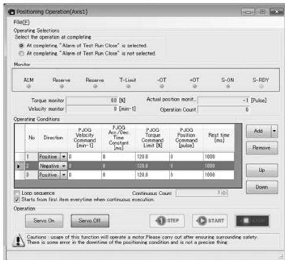
Servo motor test runs can be performed easily by issuing velocity commands and position commands from a PC. (Shows position jog operation)
