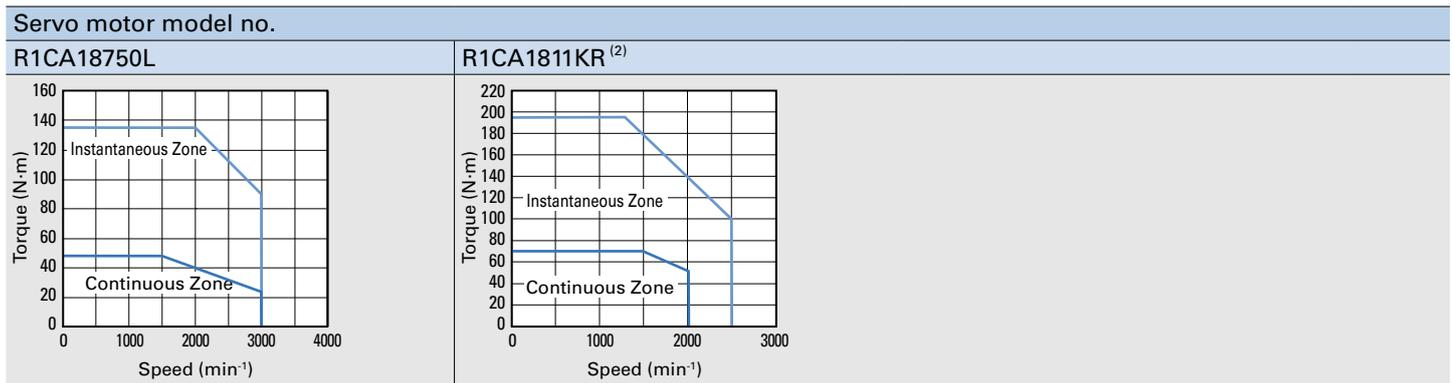
(2) Operate a motor so that the average speed does not exceed its maximum speed in the continuous zone.
