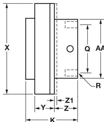
**End of Shaft - Type JD (with Actuating Disc)**
