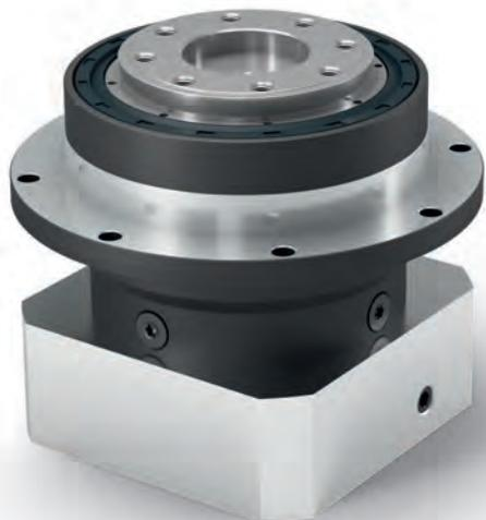
The **PFHE** represents an economically attractive alternative for high-load applications in which high radial loads occur. The combination of special pre-stressed inclined roller bearings and a flanged output shaft in accordance with ISO 9409-1 gives the **PFHE** a very high load capacity. Thanks to the radial shaft seal that is used, this gearbox achieves protection class IP65 at the output side and can therefore also withstand adverse usage conditions.
