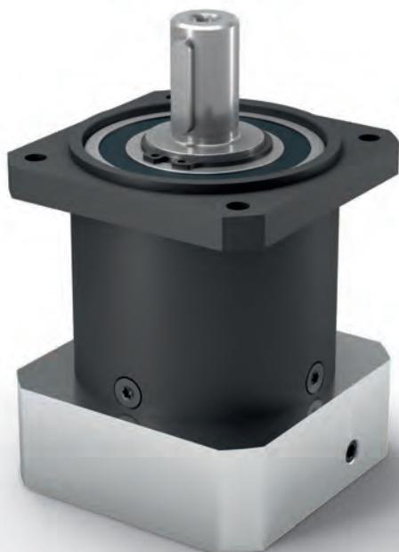
Our **PLQE** is uncomplicated and powerful. It can be connected directly to your installation without the need for an intermediate flange. The larger deep groove ball bearings on the output allow higher axial and radial forces to be absorbed. Thanks to its favorable efficiency, this means that it always operates reliably even when production cycles are demanding.
