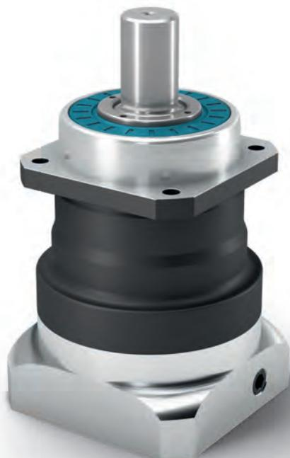
Our precision straight-toothed planetary gearbox is designed for maximum power and torque. The preloaded tapered roller bearings in the **PLN** and the specially matched seal guarantee optimum performance even in applications where dust and water spray are encountered.
