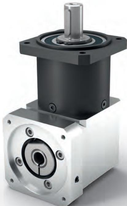
Our **WPLQE** is the right-angle gearbox with a square output flange. This makes it particularly easy to mount, versatile and, thanks to its larger deep groove ball bearings, also suitable for higher radial and axial forces.
