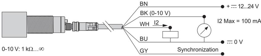
Wiring scheme (analog output 4-20 mA and PNP, NO or NC)
