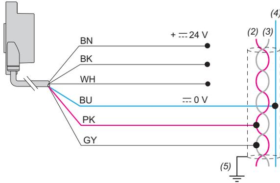
(1) Connecting the detector to the **XXZBOX01** configuration interface with the **XZCC12MDM40B** connector: BN (Brown), WH (White), BU (Blue), BK (Black).
