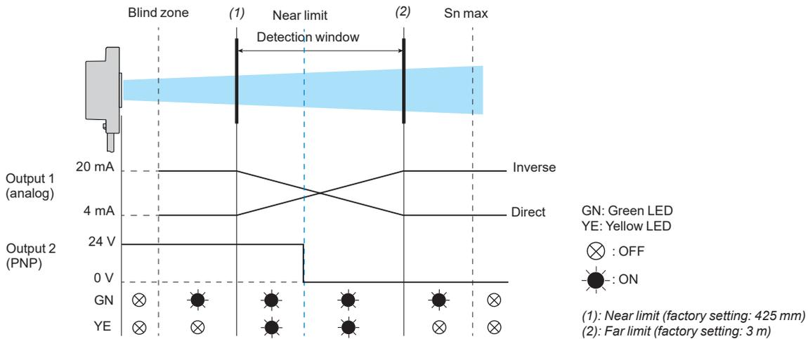
Note: The sensor's analog output emits 2 mA when it detects excessive environmental noise.
