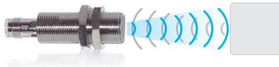
The XXV ultrasonic sensor is a “Plug and Play” solution with no adjustment or teaching required. Its solid-state output changes state when an object is less than 50 mm away from the sensor face.
