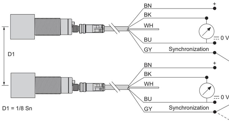
**NB:** To enable synchronization between several sensors, all of the wires of pin no. 5 (gray) must be electrically connected together. A maximum of 8 sensors can be synchronized. To enable "Multiplexer" function for the sensors, use the XX Configuration Software. Without synchronization or multiplexing, the sensors must be at least 50 cm away from each other in order to avoid mutual interference.
