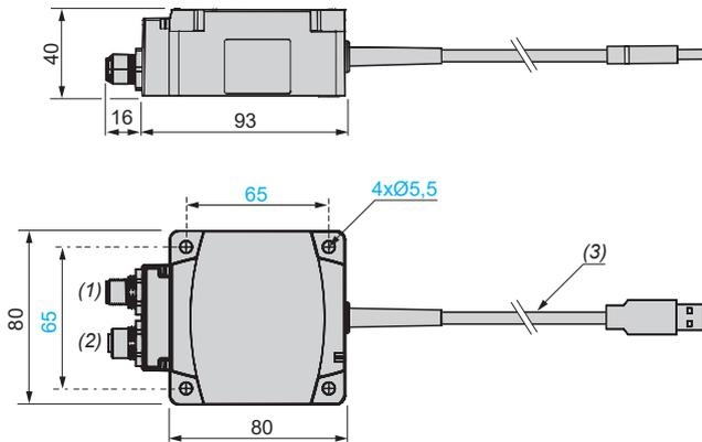
(1) Male M12 connector, 5-pin: power supply
