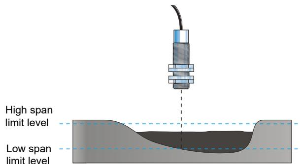
**Dual level high-low latch control detection**
