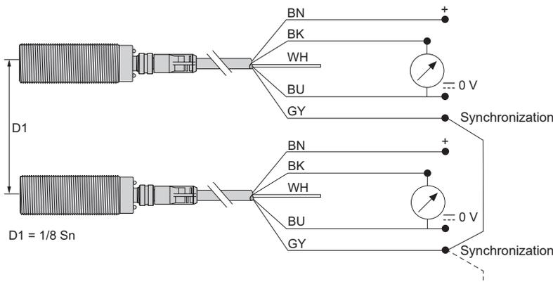
**NB:** To enable synchronization between several sensors, all of the wires of pin no.5 (gray) must be electrically connected together. A maximum of 8 sensors can be synchronized. To enable "Multiplexer" function for the sensors, use the XX Configuration Software. Without synchronization or multiplexing, the sensors must be at least 50 cm away from each other in order to avoid mutual interference.
