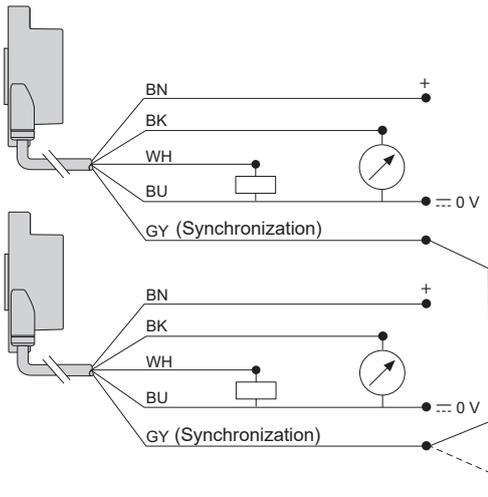
**Note:** Synchronization is recommended if more than one sensor is used in the same direction in order to avoid any interference between sensors due to the width of their beam.
