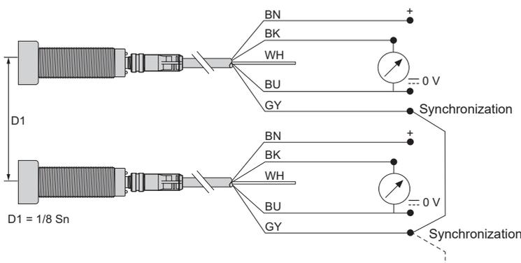
**NB:** To enable synchronization between several sensors, all of the wires of pin no. 5 (gray) must be electrically connected together. A maximum of 8 sensors can be synchronized. To enable "Multiplexer" function for the sensors, use the XX Configuration Software. Without synchronization or multiplexing, the sensors must be at least 50 cm away from each other in order to avoid mutual interference.
