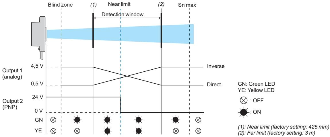
Note: The sensor's analog output emits 5 volts when it detects excessive environmental noise.
