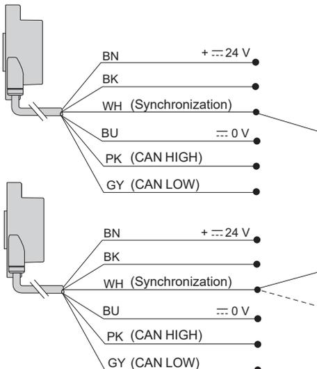
**Note:** Synchronization is recommended if more than one sensor is used in the same direction in order to avoid any interference between sensors due to the width of their beam.
