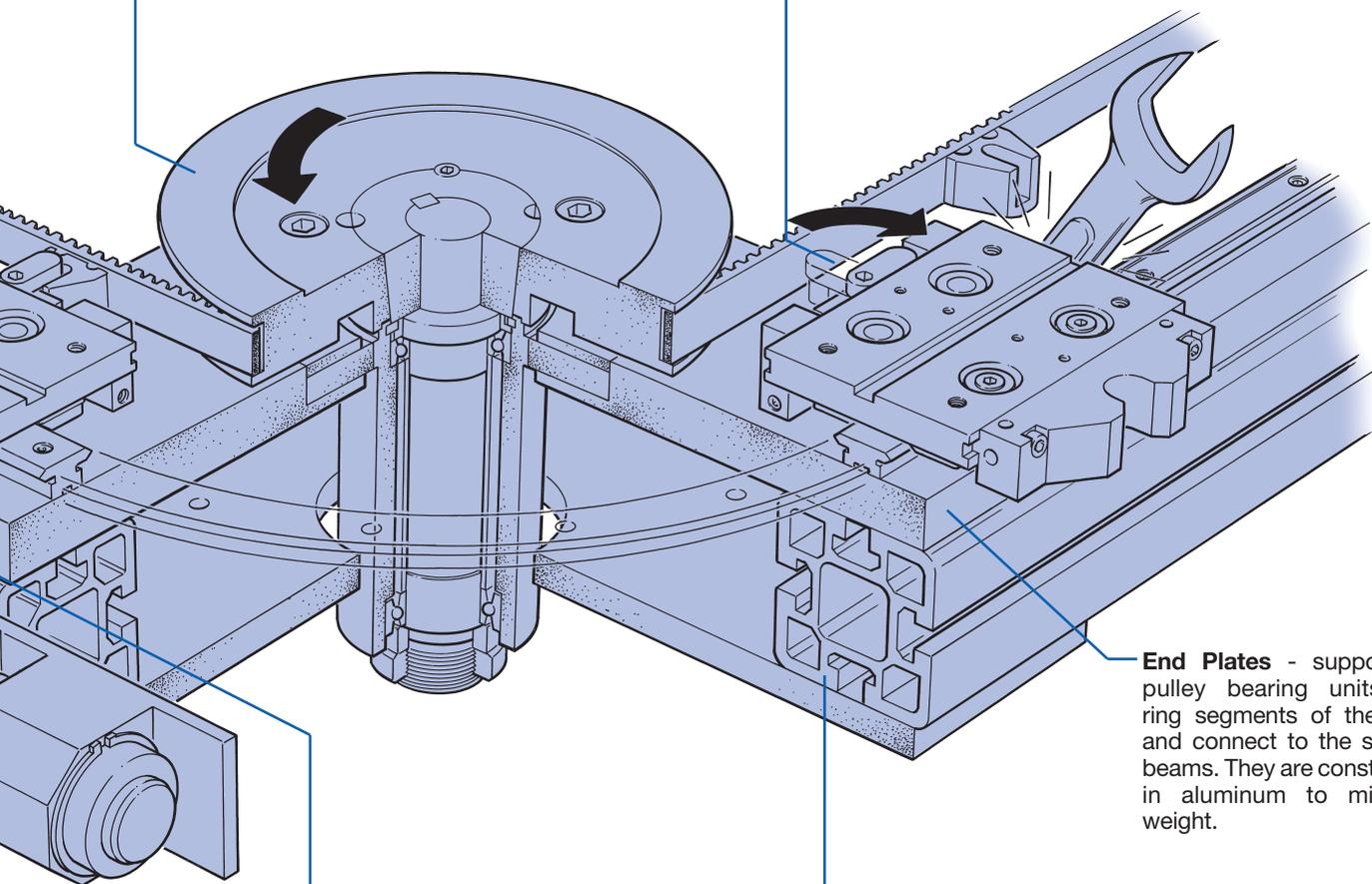
**End Plates** - support the pulley bearing units and ring segments of the track and connect to the support beams. They are constructed in aluminum to minimize weight.
