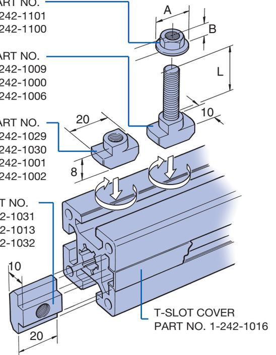
\* L is the minimum protrusion of the T-Bolt stud above the aluminum profile.
