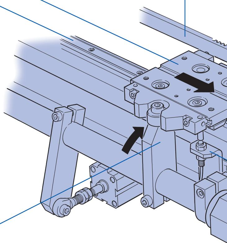
**Carriage Locking System (optional with intermittent motion):** Aligns specific carriages to a repeatable position anywhere along any straight section of the circuit to  $\pm 0.05$  mm.
