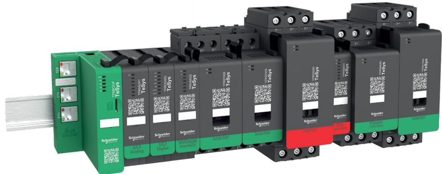
The external communication with the automation environment is made via a single coupler module, and the island is seen as a single node on the network. The other modules include starters, power interface modules, analog and digital I/O modules, voltage interface modules, and SIL interface modules, covering a wide range of operational functions.
