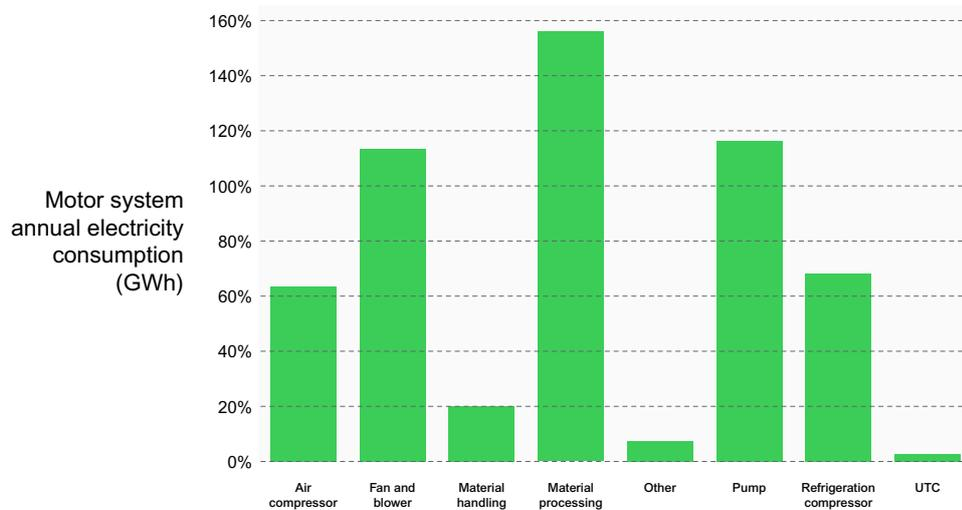
Industrial motor system annual electricity consumption by driven equipment. UTC indicates that the equipment driven by the motor could not be identified.<sup>2</sup>
