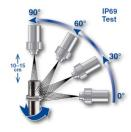
Devices bearing the IP69 rating can be used in applications in which they are exposed to high pressure (1450psi) and high temperature (175°F) wash down
