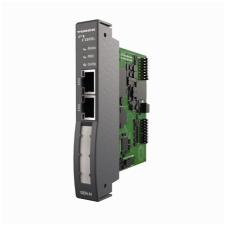
The gateway is used to connect the excom system to a higher-level Ethernet Fieldbus with the help of the Modbus TCP, Ethernet/IP and PROFINET protocols. The connection to the Fieldbus is created via a standard RJ45 male connector with at least CAT5e cable quality. A ring topology in accordance with DLR or MRP can be implemented using the built-in switch.
