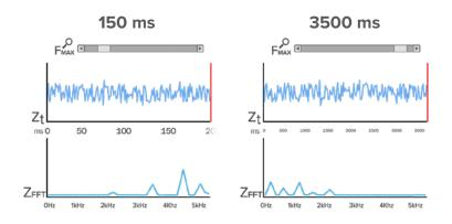
The QM30VT3 offers advanced tools like adjustable Frequency Max (FMax) and High-Frequency Enveloping mode (HFE) for applications requiring in-depth vibration analysis. Adjusting FMax lets users tailor the frequency range and sample length to machine speed and fault characteristics. Higher FMax captures a broad frequency range, using shorter sample times and default resolution suitable for detecting faults
