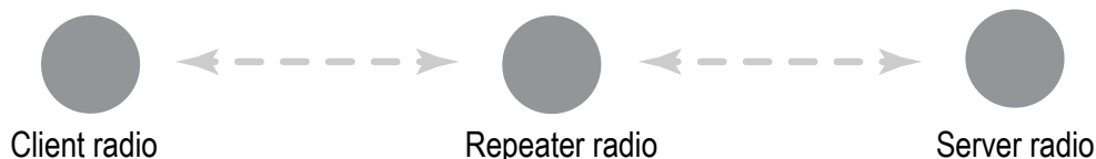
Point-to-point network with repeater for cable replacement applications
